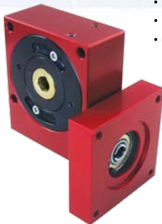
PF-NM Wormgear Reducer ≤4' Backlash up to 3,000 RPM Input 5:1 to 120:1 Ratios
