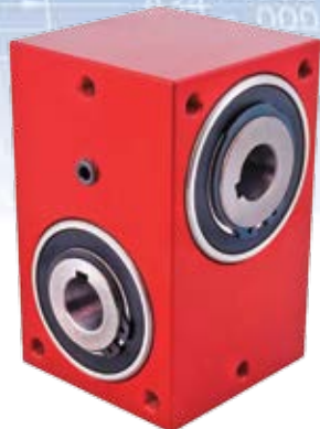
E & EA Cross Axis ≤30' Backlash up to 4,000 RPM Input 6mm to 30mm Shafts 1:1 to 40:1 Ratios
