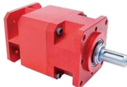
EHD Epicyclic Servo ≤30' Backlash Up to 380 Nm Torque 3:1 to 36:1 Ratios
