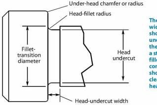
The head is the widest part of a shoulder screw. An undercut under the head permits a stress-relieving fillet while allowing components on the shoulder to mate cleanly with the head.
