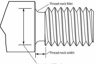
Shoulder screws' threaded regions are usually fairly short. An undercut or neck slightly smaller than the thread minor diameter joins the threaded region to the shoulder.
