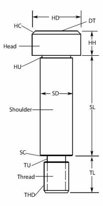
*Head diameter.* The head diameter is the largest diameter of the screw, typically twice the head height and 30 to 50% larger than the shoulder diameter. Head-diameter tolerances run  $\pm 0.005$  in. for inch screws and  $\pm 0.127$  mm for metric sizes. For commercial-grade screws, manufacturers or users sometimes add a straight knurl on the head diameter.
