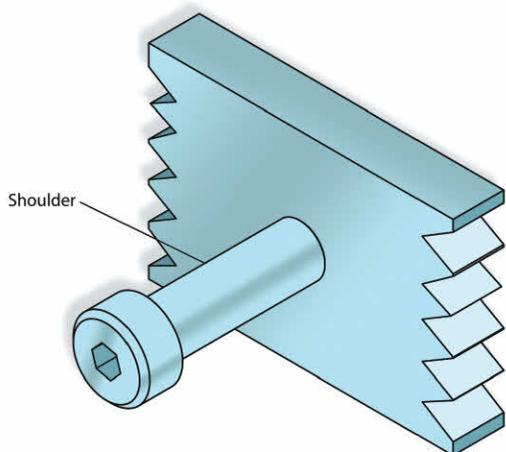
When the thread of a shoulder screw is fully installed, the unthreaded shoulder stands proud of the surface. It can work as journal for rotating parts or a guide for sliding parts, among many other possibilities.
