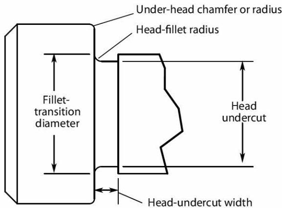
The head is the widest part of a shoulder screw. An undercut under the head permits a stress-relieving fillet while allowing components on the shoulder to mate cleanly with the head.
