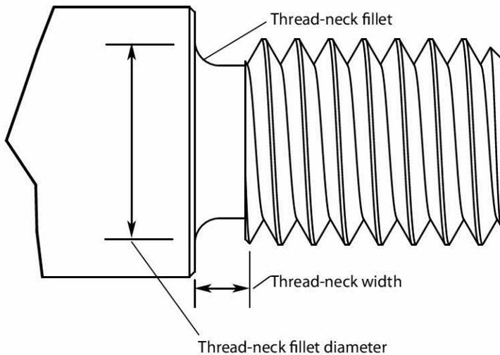
Shoulder screws' threaded regions are usually fairly short. An undercut or neck slightly smaller than the thread minor diameter joins the threaded region to the shoulder.
