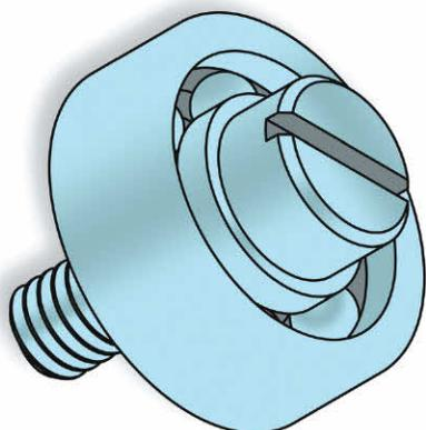
To create a simple cam follower, mount a ball bearing on a shoulder screw. With proper shoulder length and tolerances, the screw can fix the inner race of the ball bearing while still allowing the outer race to spin freely.
